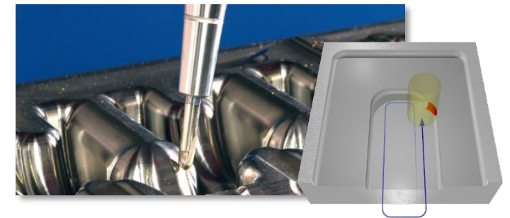
Fig. Milling process for machining molds using a ball end mill [ISF] .
